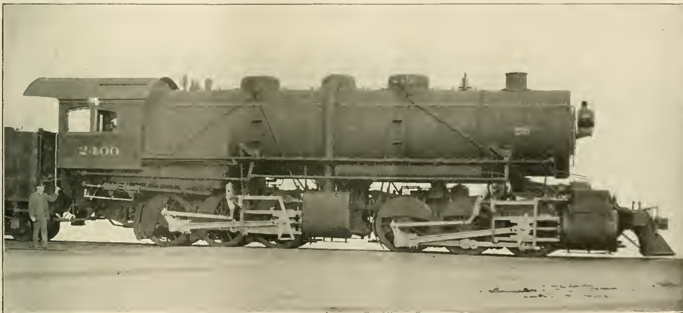
MALLET 4-CYLINDER ARTICULATED COMPOUND FOR THE B. & O.
